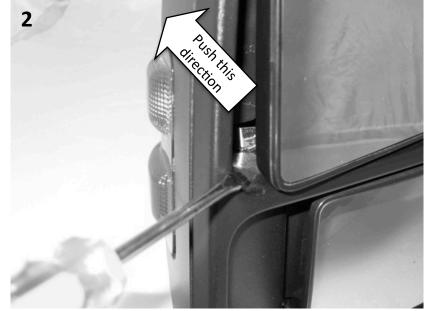
2. Using a flat screwdriver, push the tab into the turn signal to release the turn signal lens.
