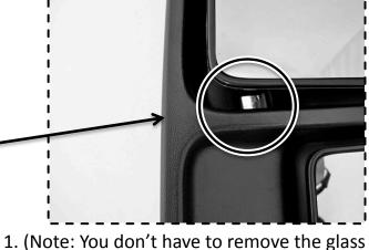
1. (Note: You don't have to remove the glass or the mirror assembly from the truck to complete this installation.) Pull the glass holder up from this corner to see the silver plastic tab underneath. (LH mirror is used in
